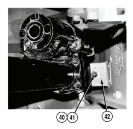
16. Remove switch (40) and washer (41) from bracket (42).
