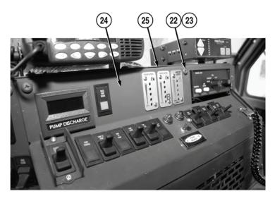
15. Install cab instrument panel B (24) on cab instrument panel assembly (25) with five lockwashers (23) and screws (22).
