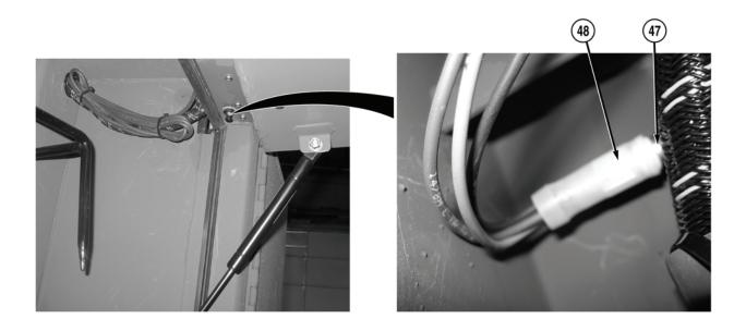
9. Connect driver side body wire harness connector (47) to driver side center stowage compartment D2 door switch (48).
