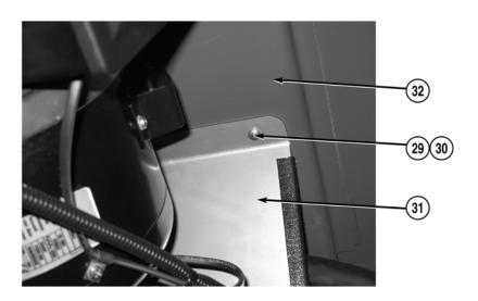
11. Remove two screws (29), washers (30), and heat shield (31) from rear storage compartment (32).
