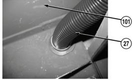
42. Remove passenger side body wire harness (27) from vehicle.
