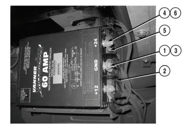
4. Install cable (5) on terminal (6) with locknut (4).
