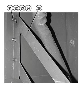
14. Install shelf support (28) on vehicle with three screws (34), six washers (33), three lockwashers (32), and nuts (31).
