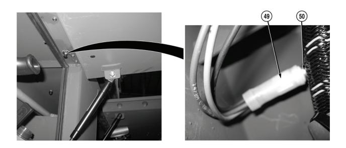
8. Connect driver side body wire harness connector (49) to driver side front center stowage compartment D3 door switch (50).
