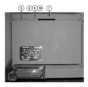
3. Remove four locknuts (8), eight washers (9), four screws (10), and two hinges (5) from cover (7). Discard locknuts.
