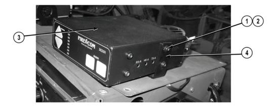
1. Remove four screws (1), washers (2), and intercom (3) from bracket (4).
