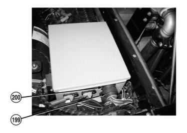
58. Disconnect pump power distribution connector DP 2 (199) from pump house distribution box DP 2 connector (200).
