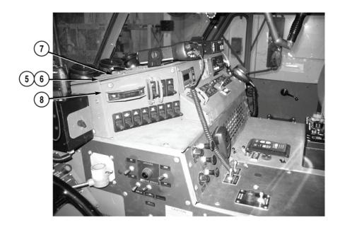
3. Remove seven screws (5) and lockwashers (6) from instrument panel A (7). Discard lockwashers.
