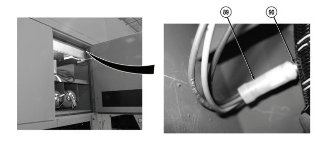
7. Connect passenger side body wire harness connector (89) to passenger side center stowage compartment P2 door switch (90).
