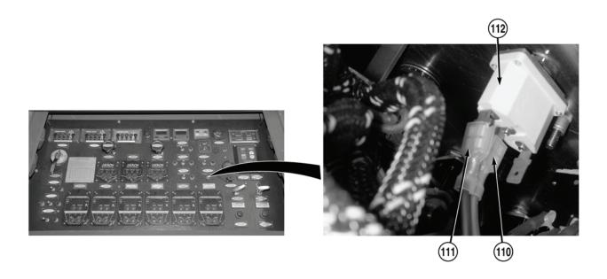
35. Connect wire 2346 (110) and wire 1661 (111) to PANEL LIGHTS switch (112).
