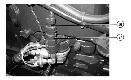
9. Connect water pump engine wire harness connector (26) to oil pressure sending unit (27).
