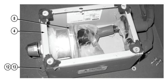
4. Remove battery disconnect switch (8) from battery disconnect box (4).
