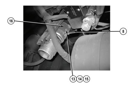
5. Remove two locknuts (13), four washers (14), two screws (15), and clamp (16) from water pump engine oil drain mounting bracket (8). Discard locknuts.
