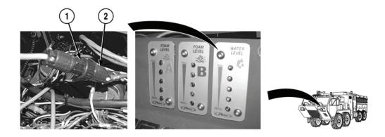
3. Connect cab water tank level indicator gauge connector (2) to cab water tank level indicator wire harness connector (1).
