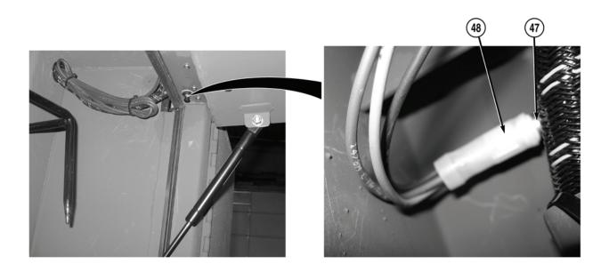
23. Disconnect driver side body wire harness connector (47) from driver side center stowage compartment D2 door switch (48).
