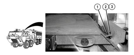
4. Repair two wires (2) and (3) and close loom (1) (TM 9-2320-325-14&P).
