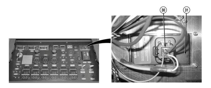
8. Disconnect pump operator's panel wire harness connector (30) from ENFO IV display module (31).
