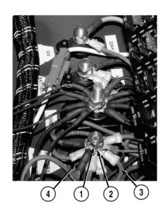
16. Install eight wires 1138 (3) on cab 24 VDC terminal block (4) with lockwasher (2) and nut (1).
