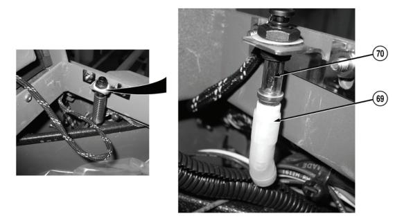
26. Disconnect passenger side body wire harness connector (69) from rear passenger side top stowage compartment door switch (70).
