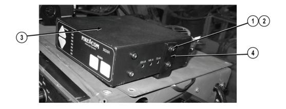
11. Install intercom (3) on bracket (4) with four washers (2) and screws (1).
