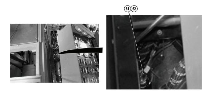
29. Connect main wire harness connector (61) on valve control wire harness connector DV1 (62).
